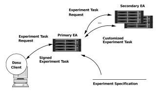
Fig. 10: Interaction between Dasu Clients and the Experiment Administration Service.
