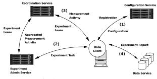
Fig. 5: Dasu system components.
