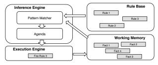
Fig. 7: Rule-based program execution environment.
