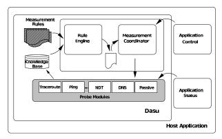
Fig. 6: Dasu client architecture.
